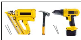
nails inflation gun / hammer + finishing nails (without head) / screw driving machine + self-tapping screws
